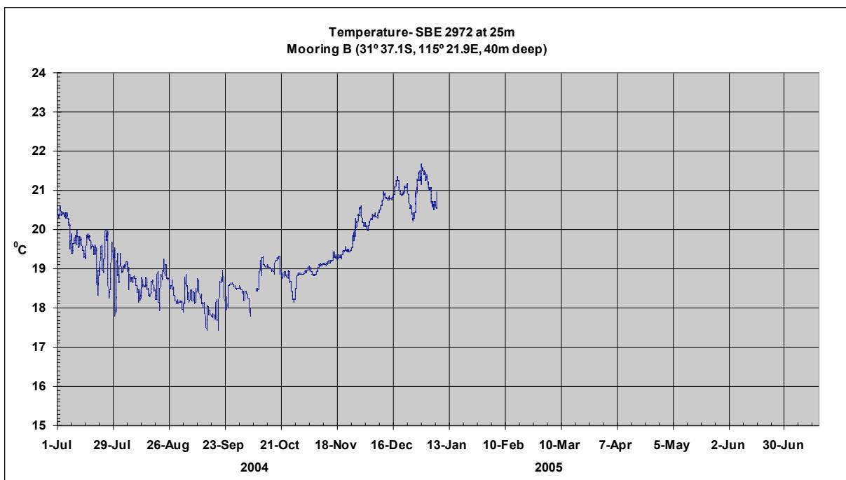
*Figure 4: Temperature at 25m depth at Site B based on hourly time-series*
