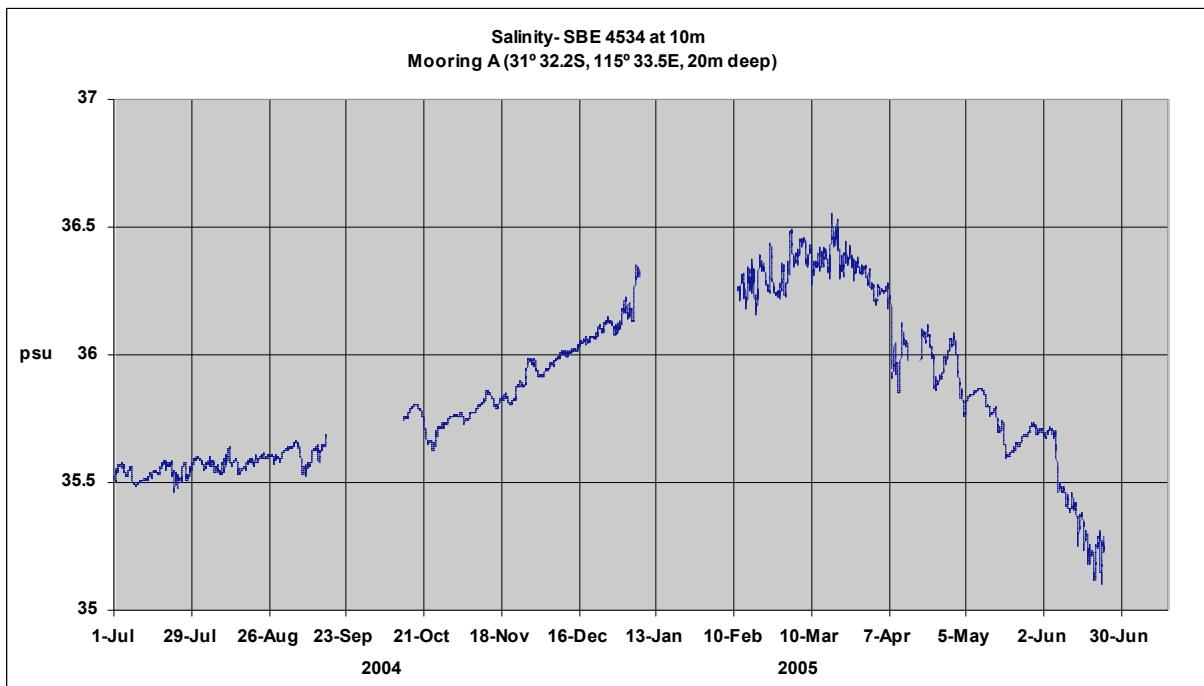
Figure 8: Salinity at 10m depth at Site A based on hourly time-series
