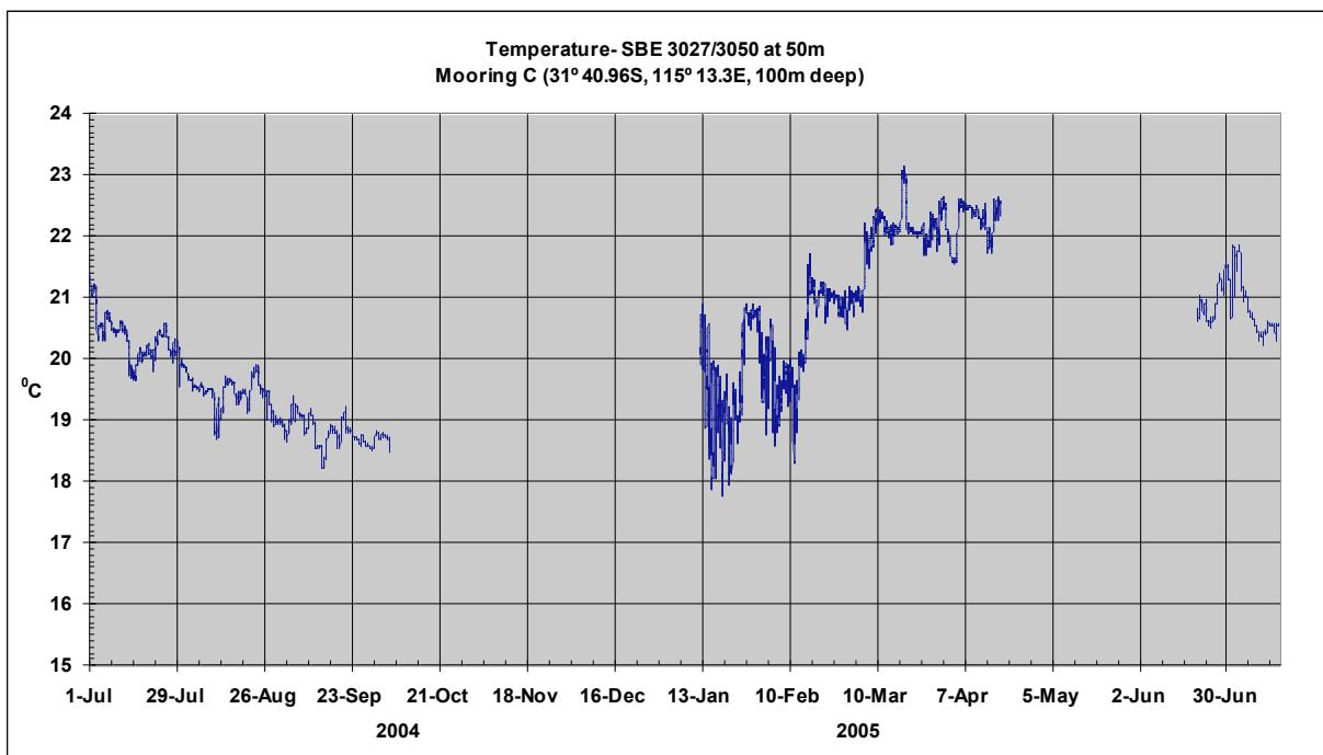
Figure 5: Temperature at 50m depth at Site C based on hourly time-series
