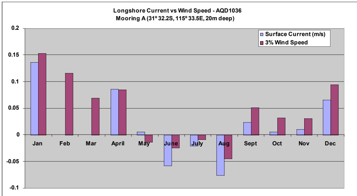
Figure 19: Long-shore current near the surface vs 3% of the long-shore component of wind speed at Site A.
