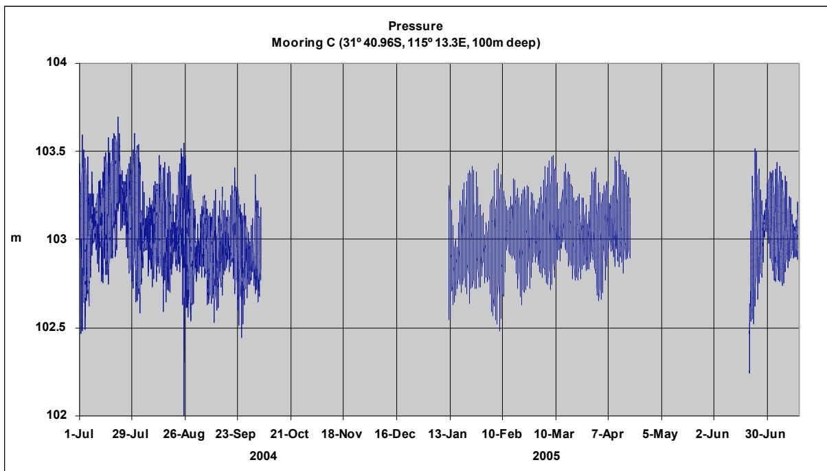
Figure 13: Pressure at the ocean bottom at Site C based on hourly time-series
