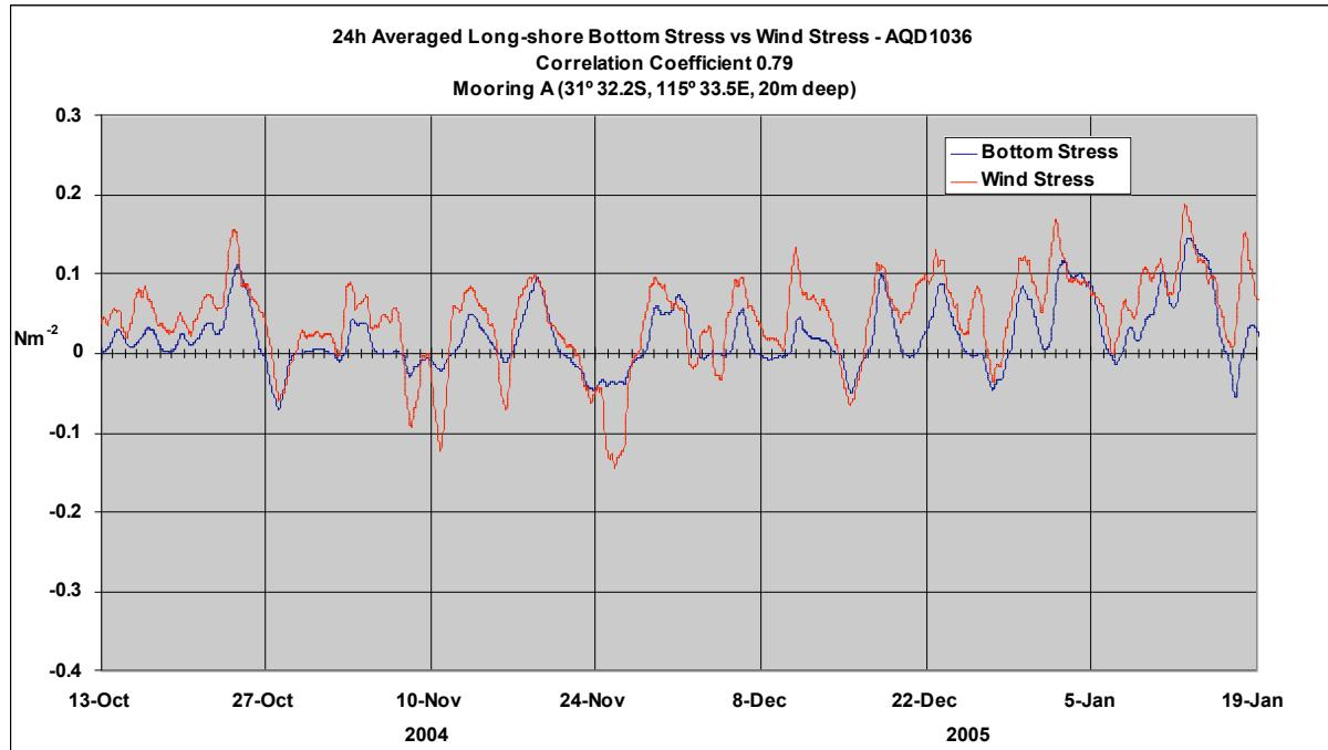
Figure 16: 24hr-averaged long-shore quadratic bottom stress (based on depth averaged current) vs long-shore wind stress at Site A from 13 Oct 2004 to 19 Jan 2005
