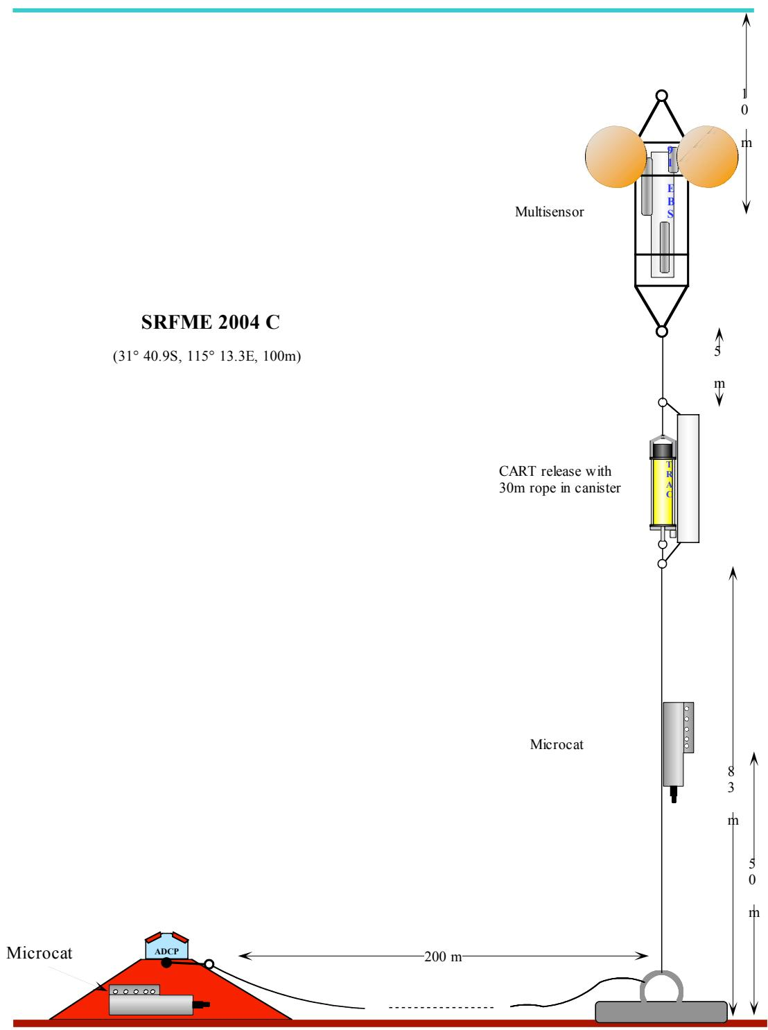
Figure 26: Mooring C, where the Multisensor is SBE 4536, the Microcats are SBE 3027 and 3050 and the ADCP is RDI 3712 or 3713.
