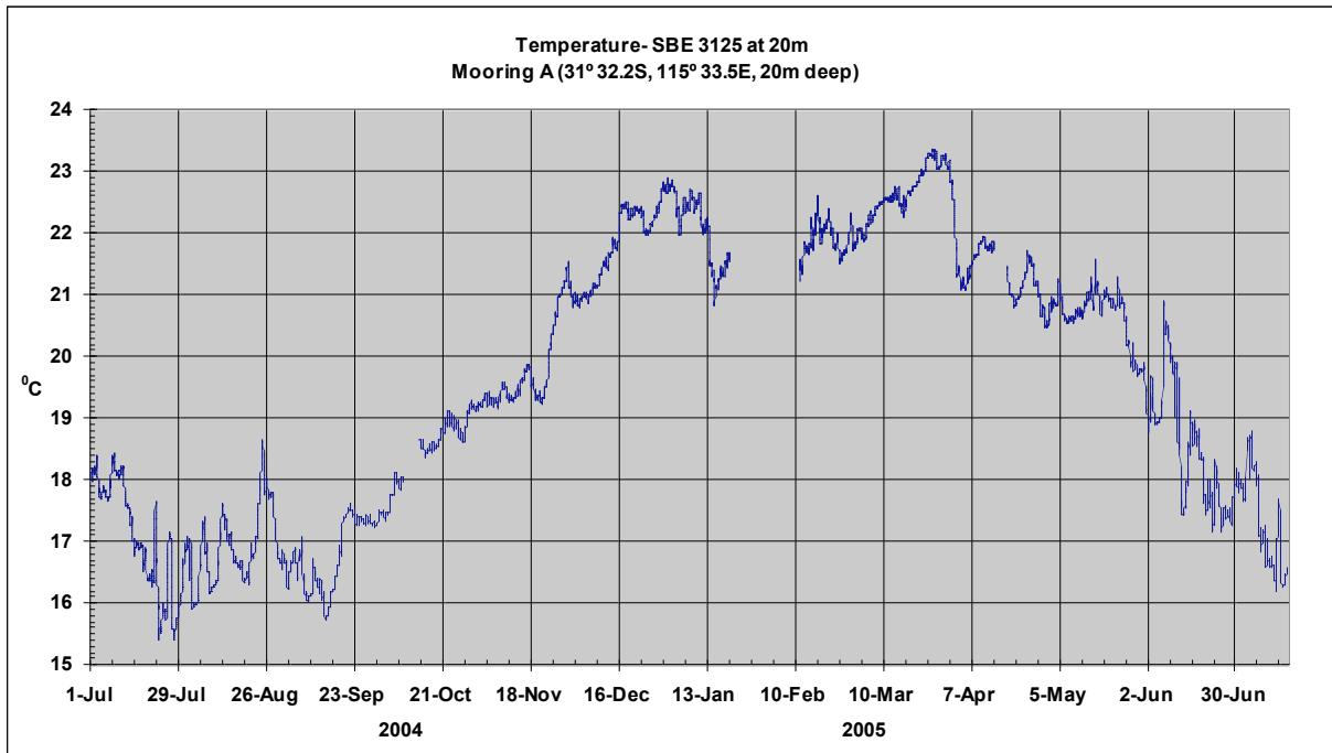
*Figure 3: Temperature at 20m depth at Site A based on hourly time-series*
