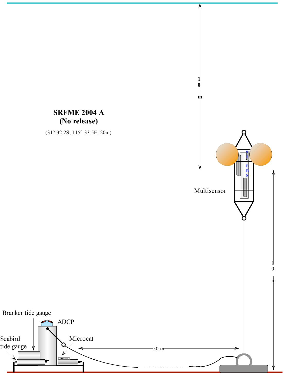
Figure 24: Mooring A, where the Multisensor is SBE 4534, Microcat is SBE 3125 and ADCP is AQD 1036. No data was collected by the Branker tide gauge.
