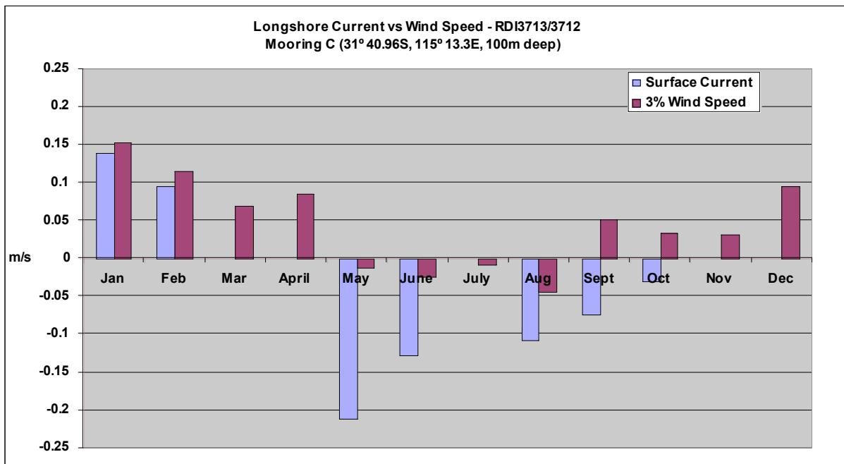
Figure 20: Long-shore current near the surface vs 3% of the long-shore component of wind speed at Site C
