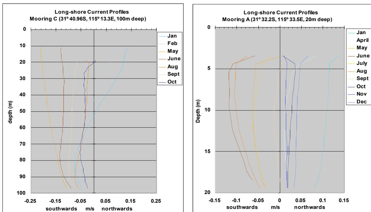
Figure 18: Monthly-averaged long-shore current profiles at Sites C and A
