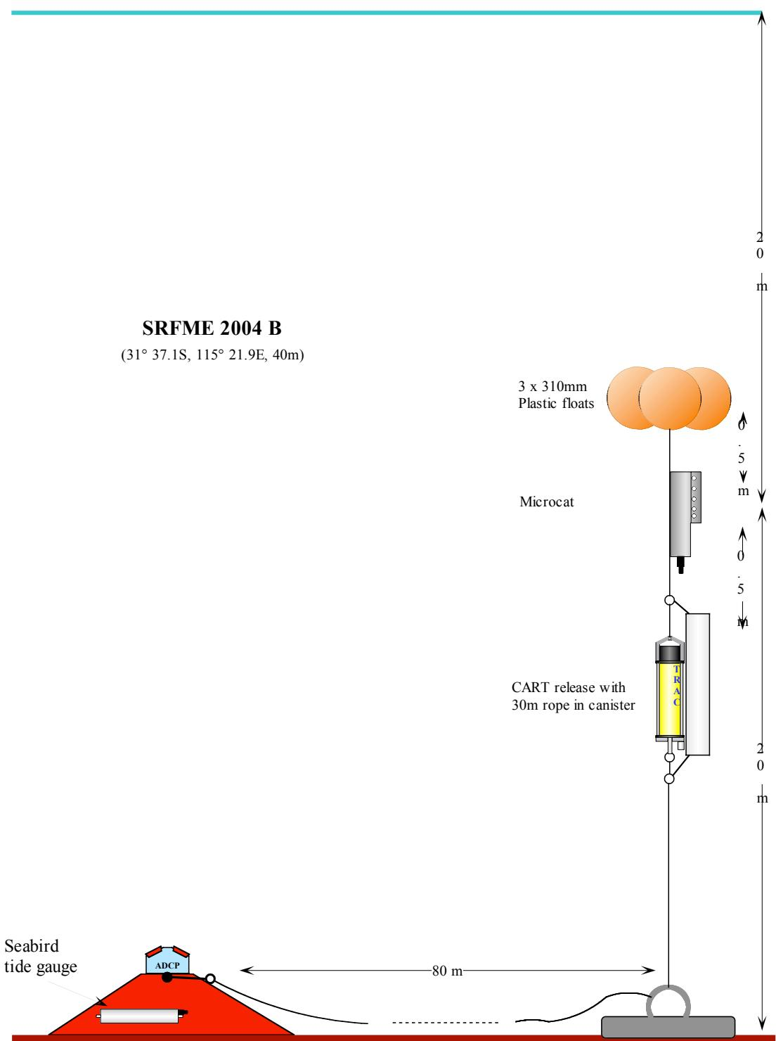
Figure 25: Mooring B, where the Microcat is SBE 2972 and ADCP is RDI 3712 (no data due to failure) and RDI 3713. No data was collected by the Seabird tide gauge.
