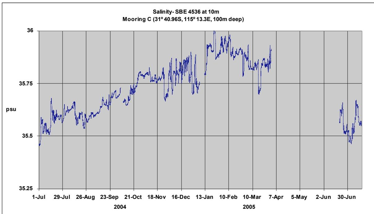
Figure 11: Salinity at 10m depth at Site C based on hourly time-series
