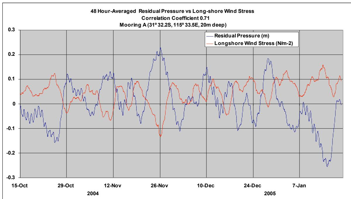
Figure 17: 48hr-averaged residual pressure vs long-shore wind stress at Site A from 15 Oct 2004 to 19 Jan 2005
