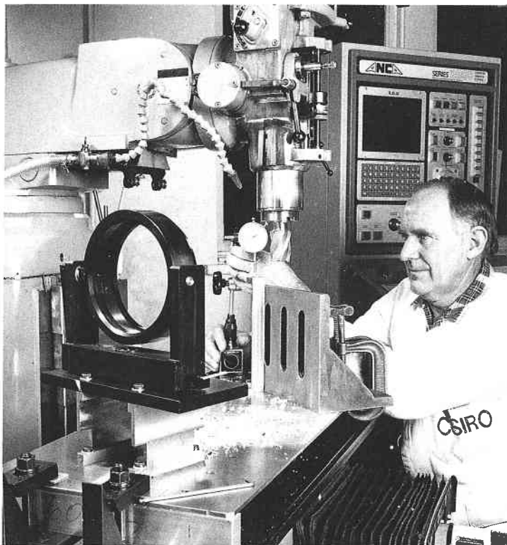
Construction of the optical housing of the prototype Atmospheric Pressure Scanner on a computer controlled mill in the Division workshop.
