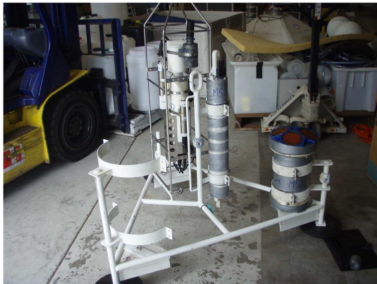
Figure 16 MS1 mooring showing SBE19p (left), SBE26 (middle) and RDI ADCP (right).
