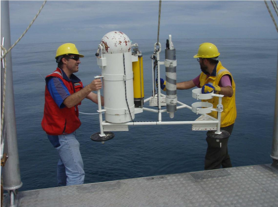
Figure 21 Deploying MS2 showing acoustic release and SBE26
