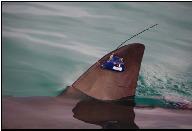
Figure 19. A SAT tag correctly attached to the dorsal fin of a juvenile white shark (image courtesy of George Trinkler).
