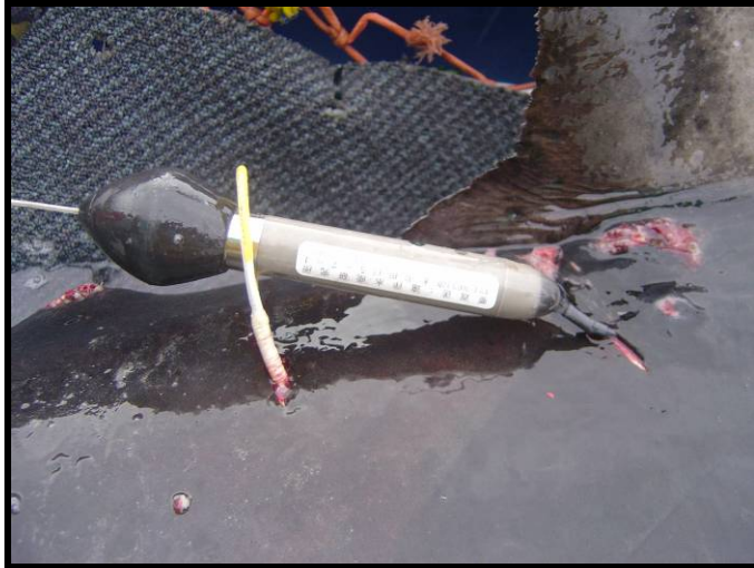
Figure 16. PSAT tag with secondary anchor (to left) secured into the dorsal musculature and in-line with the primary anchor just behind the dorsal fin.
