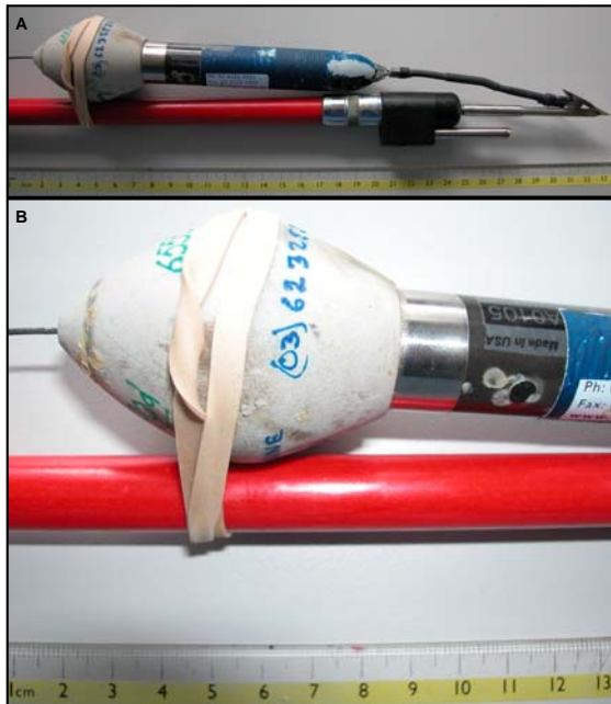
Figure 15. PSAT tag, rigged for deployment on white shark, ready for deployment. A: overview; B: detail showing rubber band placement.
