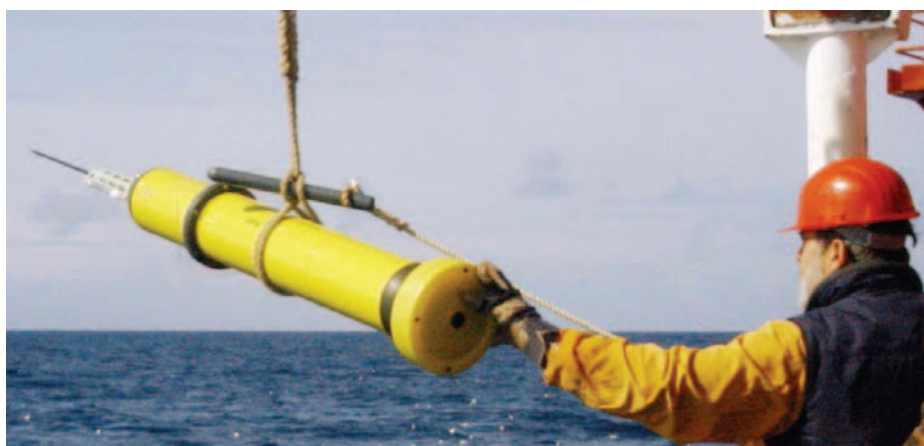
Launching floats. The temperature/salinity sensors and satellite communication antenna are at the top. The bladder that controls rise and fall of the instrument is at the bottom.
