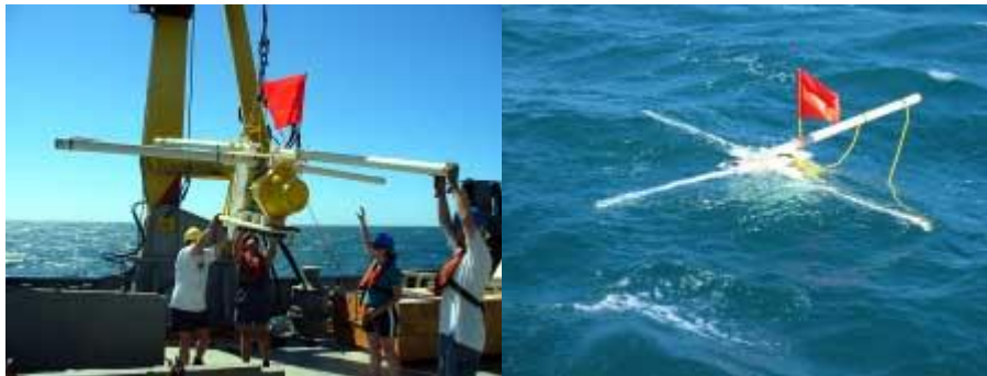
Figure 3. An OBEM about to be deployed (left). A ballast weight causes it to sink to the bottom where it remains until the weight is acoustically released and the instrument floats back up to the surface for recovery (right). A magnetometer and other electronics (including acoustics) are housed in glass spheres (inside the yellow protective container); electrodes the end of each of the white pipes allow measurement of the electric field gradient in two orthogonal horizontal directions.
