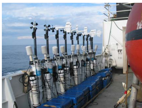
Figure 2. Surface instruments setup for system checks on the weather deck.
