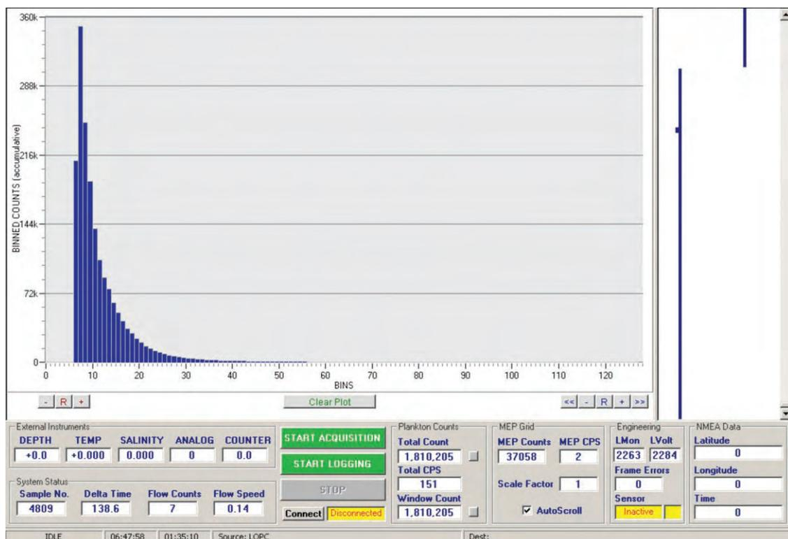
**Figure 7:** Laser Optical Plankton Counter replay after a ss2010\_v08 MOCNESS deployment, showing the number of planktonic particles counted over a wide size spectrum.
