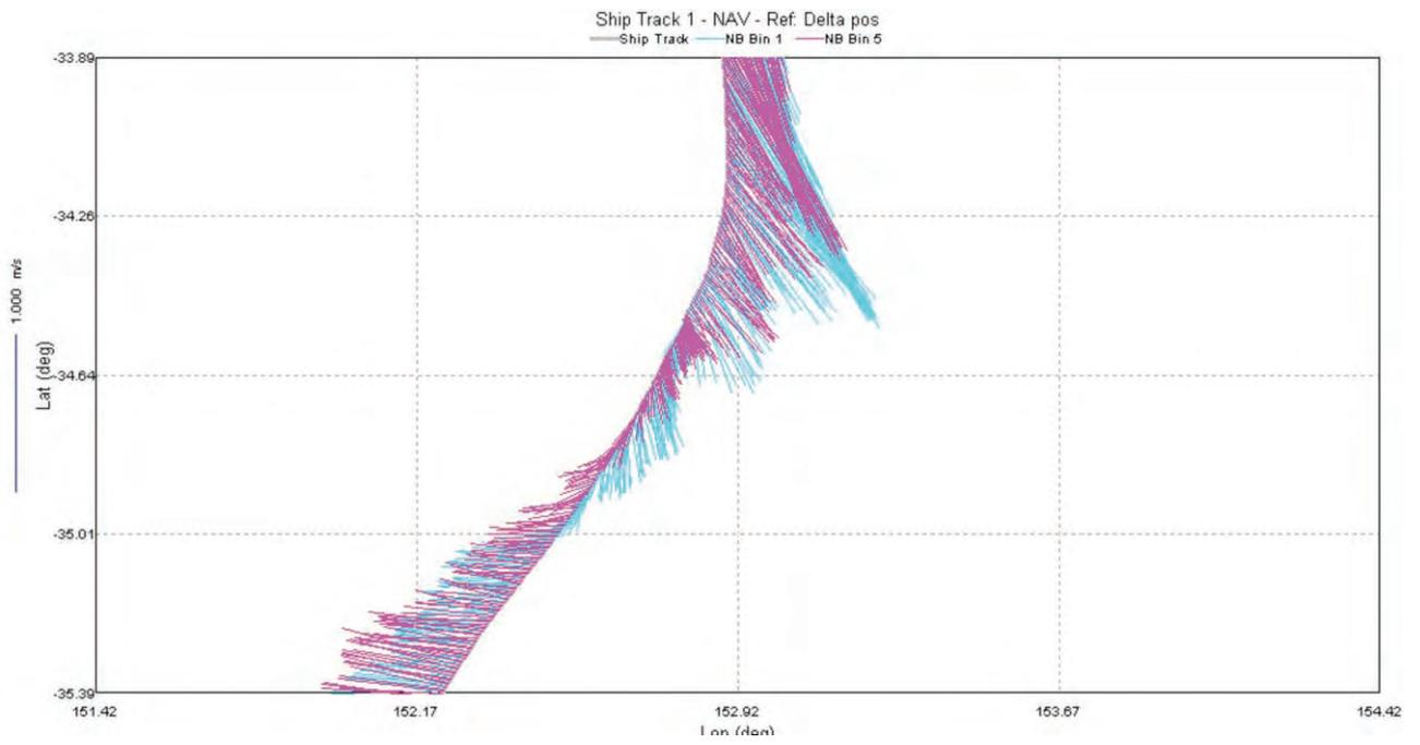
**Figure 8:** ADCP transect across cold core eddy and south into warm core eddy.
