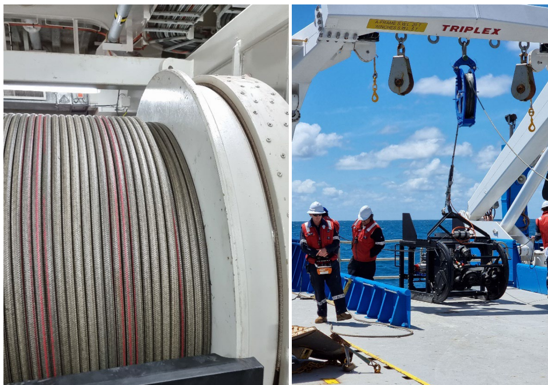
Fig 1. Deep Corer Winch line post re-spooling showing minor burying on cheekplate (left). Deep Tow Camera prepared for first deployment on HOTS (right).
