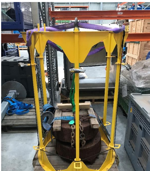
Yellow Frame Headweight 500kg – HOTS & TBW Calibrations
