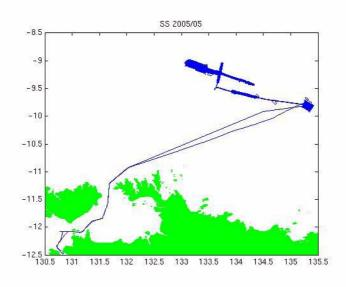
Position data was acquired using the Seapath 200 position and motion reference unit. Depth data was acquired with the Simrad EA500. The Divisional Data Librarian can assist with information regarding all other sensors.
