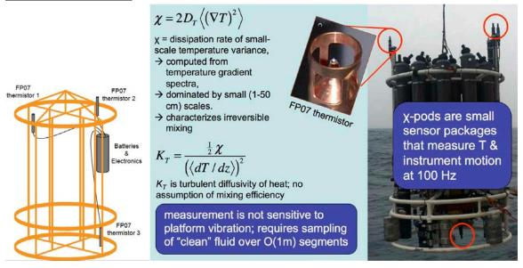
All of instruments are internally recording, and consist of a sensor 3 cm x 12 cm cabled to an electronics pressure case (7cm x 40 cm), all rated to 6000 m. Each is powered by 2 lithium batteries, which we ship directly to the ship and install there.
