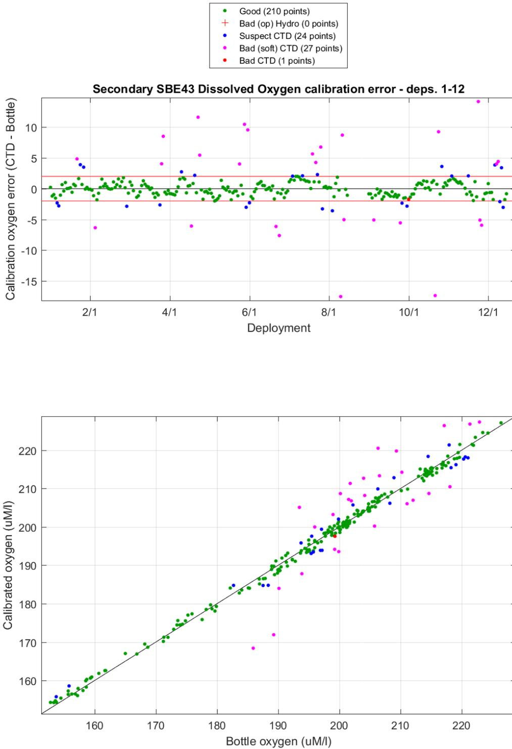
Figure 7. Dissolved Oxygen calibration, all deployments – secondary sensor
