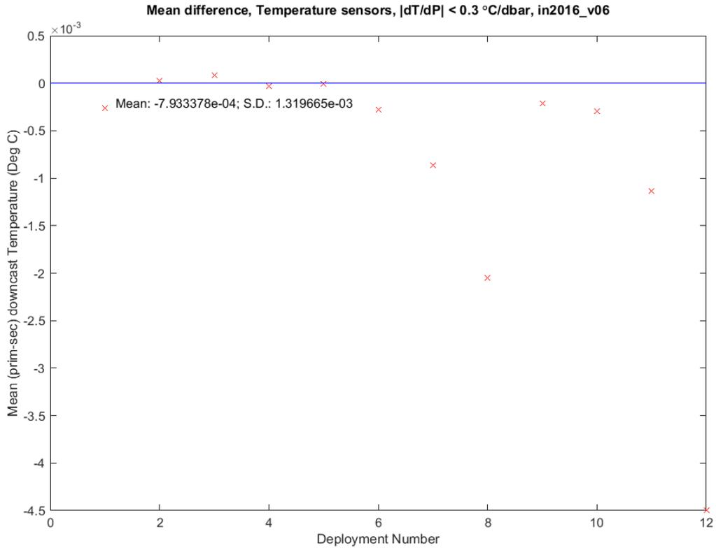
Figure 3. Temperature sensor difference
