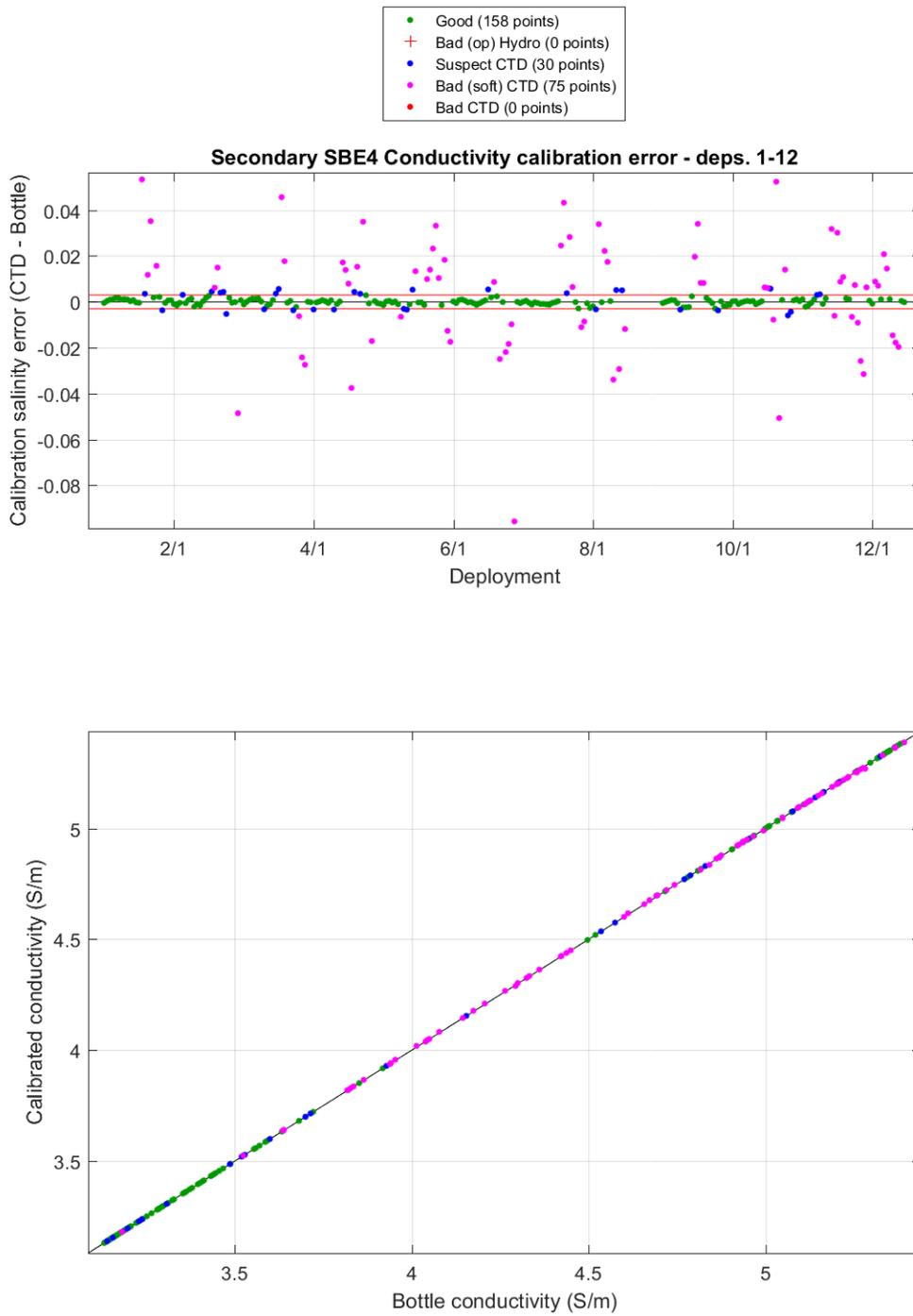
Figure 5. Secondary conductivity calibrations
