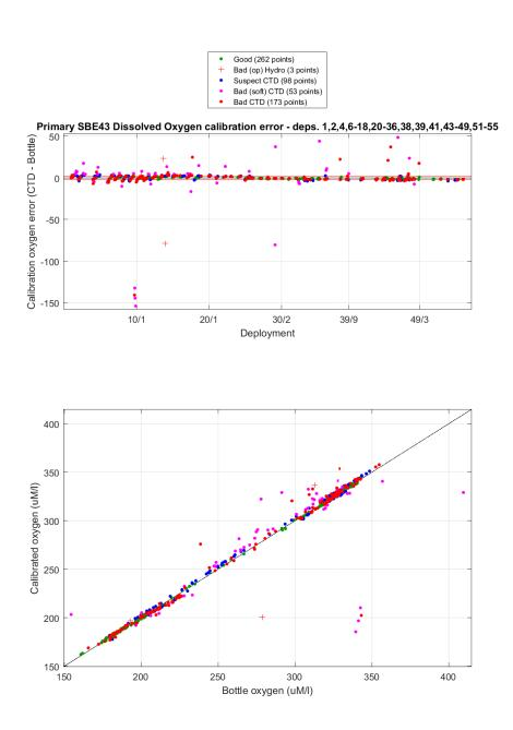
Figure 6. Dissolved Oxygen calibration, all deployments – primary sensor
