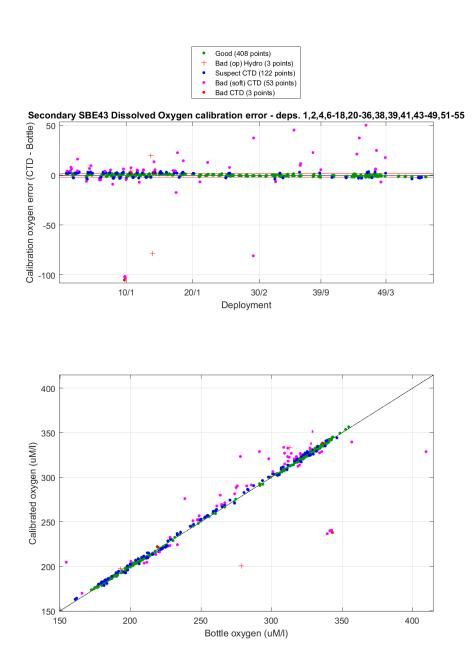
Figure 7. Dissolved Oxygen calibration, all deployments - secondary sensor
