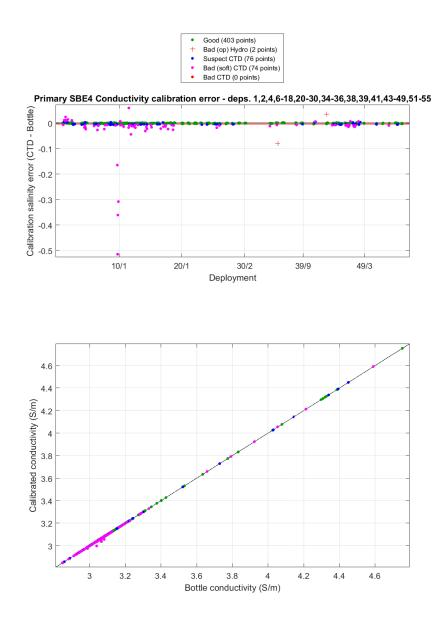
Figure 4. Primary conductivity calibrations
