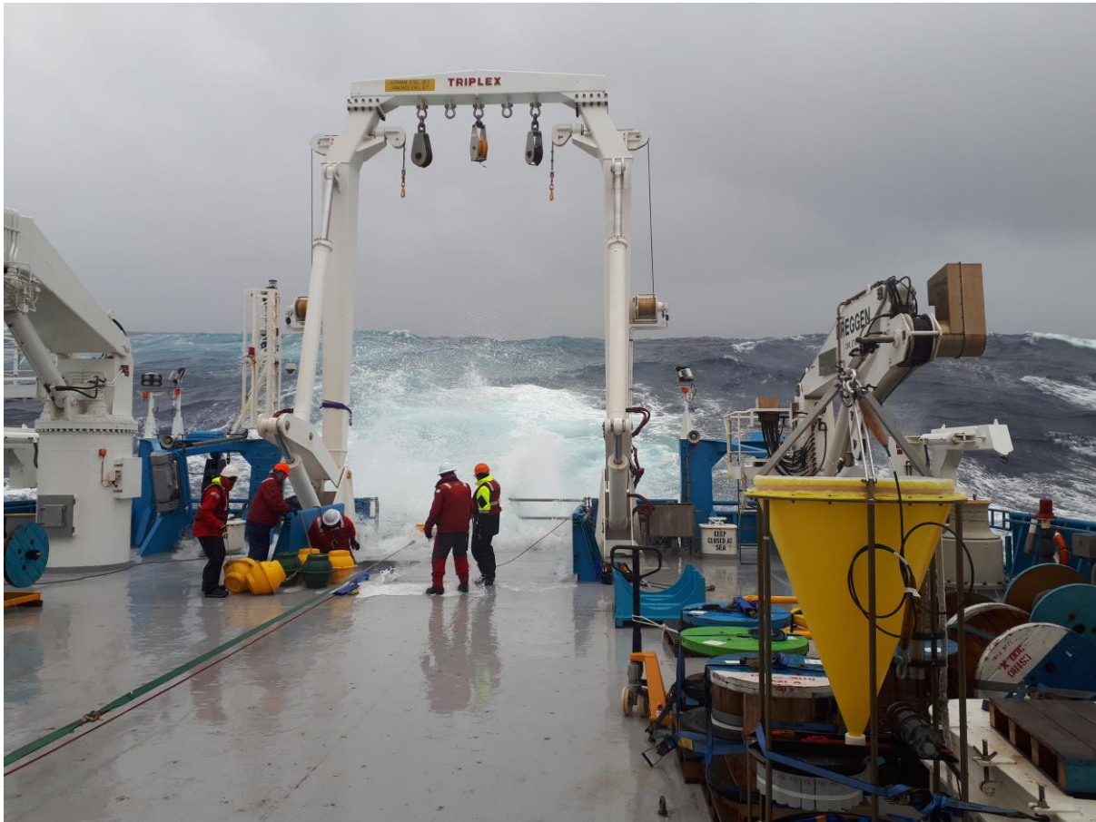
Figure 1. Working conditions at SOTS in winter – deploying the SAZ sediment trap mooring. Left to Right: Phil De Boer, Jim LaDuke, Matthew Schmierer (kneeling), James Hogg, Tim Lane, and the last sediment trap ready to go (yellow funnel). Photo Peter Jansen.
