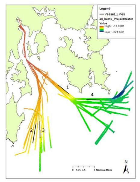
Locations of backscatter calibration lines in Storm Bay. Departing Hobart, we will either repeat line 2 or line 3 (highlighted below).
