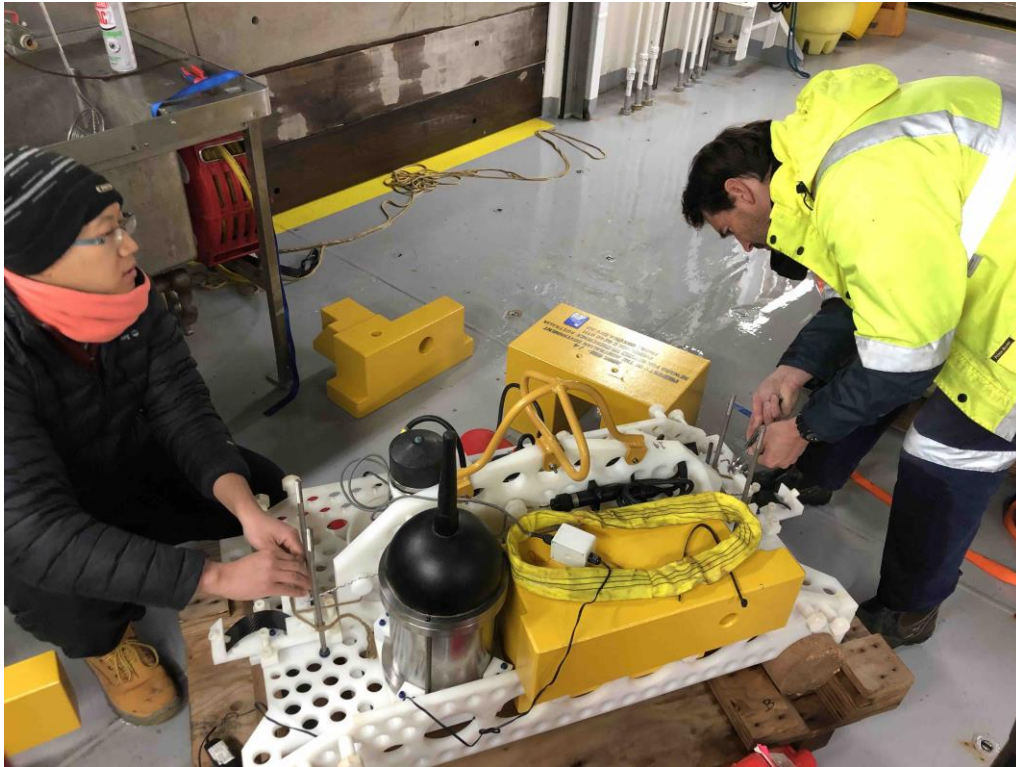
Preparing Australian Geophysical Observing System (AGOS) ocean bottom seismometers (OBS) for deployment, with RSES/ANU Dr Xiaolong Ma (left) and Andrew Latimore (right). Credit: Hrvoje Tkalić, RSES/ANU.
