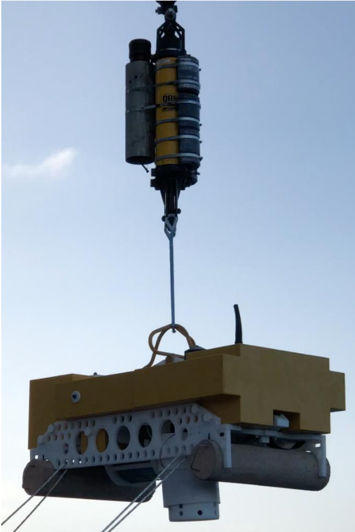
Near-bottom deployment of Australian Geophysical Observing System (AGOS) ocean bottom seismometer (OBS), with ultra-short baseline (USBL) acoustic positioning system. Credit: Hrvoje Tkalčić, RSES/ANU.
