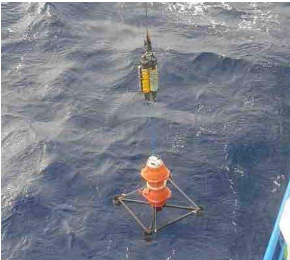
Near-bottom deployment of Chinese Academy of Sciences (CAS) ocean bottom seismometer (OBS), with ultra-short baseline (USBL) acoustic positioning system. Credit: Mike Watson, ASP.
