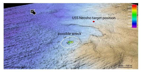
Following the *Neosho* survey, we increased speed transiting to the north-west direction to line up on the *Lexington* target position. Within 8 nm of the position we again slowed to 6 kn and maintained the same multibeam and sub-bottom profiler configuration settings. The seafloor became notably rougher with long streaks of high reflectance backscatter trending in a south-east to north-west direction, likely due to elongate rocky ridges about 100 m high exposed at the seafloor.
