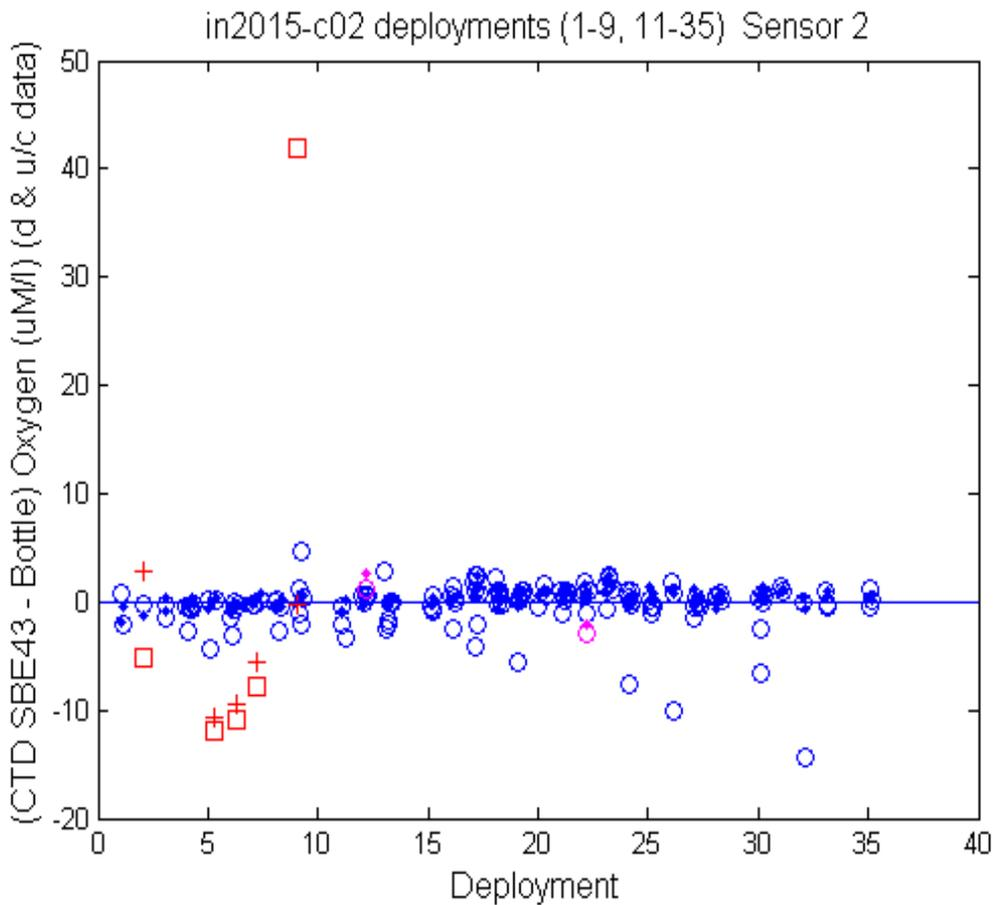
**FIGURE 7. (SBE43 - Bottle) Oxygen Difference with upcast and downcast CTD data**
