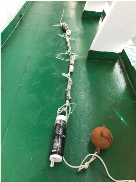
Figure 3: Thermometers on rope with metal weight (as deployed on OUC DongFangHong II).
