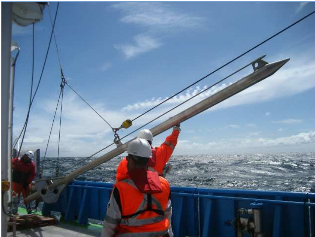
Figure 1: The FIELAX HeatFlowProbe during its deployment on board the vessel “R.V. Investigator”.
