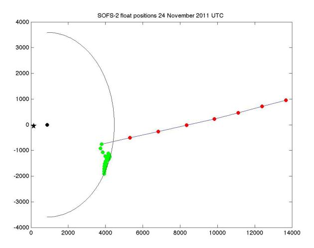
SOFS-2 buoy positions from 0200 24 November – 0800 25 November 2011 UTC. Circles indicate surface float position relative to anchor drop position. Red is while being deployed. Green is after anchor dropped. Star is anchor drop position. The arc is the expected buoy watch circle with centre at the black dot. The centre position was selected to match the buoy locations
