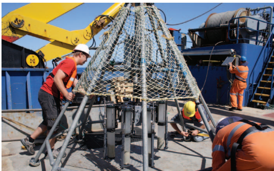
The multicorer being fixed to the rear deck after returning with sediment in the tubes. The sediment-water interface is clearly visible in several of the tubes.
