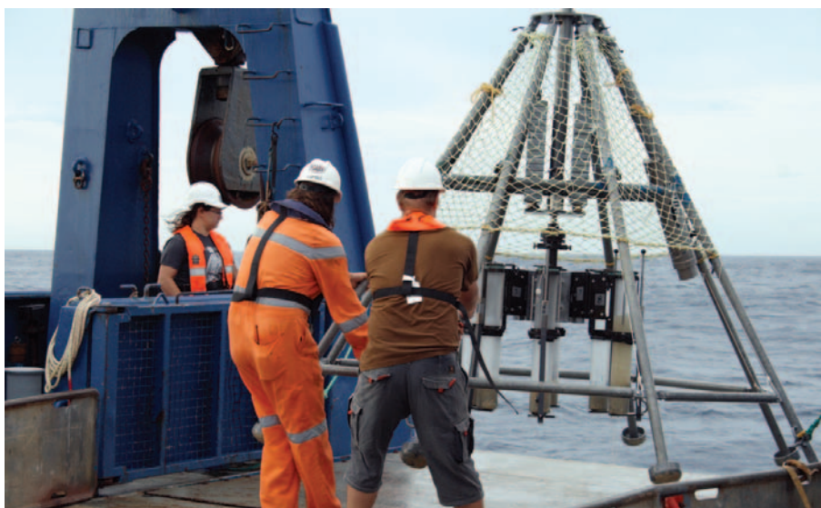
The multicorer being returned on the rear deck with sediment in the lower half of the tubes. The entire apparatus weights about 800 kilos.
