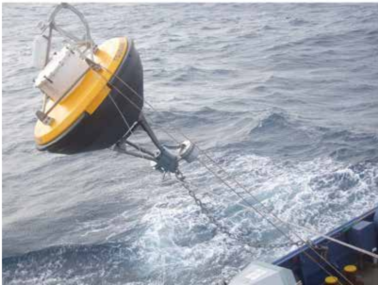
Top left: ETD (Easy To Deploy) Buoy and (above) BPR (Bottom Pressure Recorder) being deployed.
