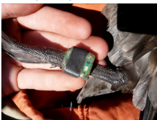
Fig 2. Mk-19 GLS tag and attachment on an adult shearwater.
