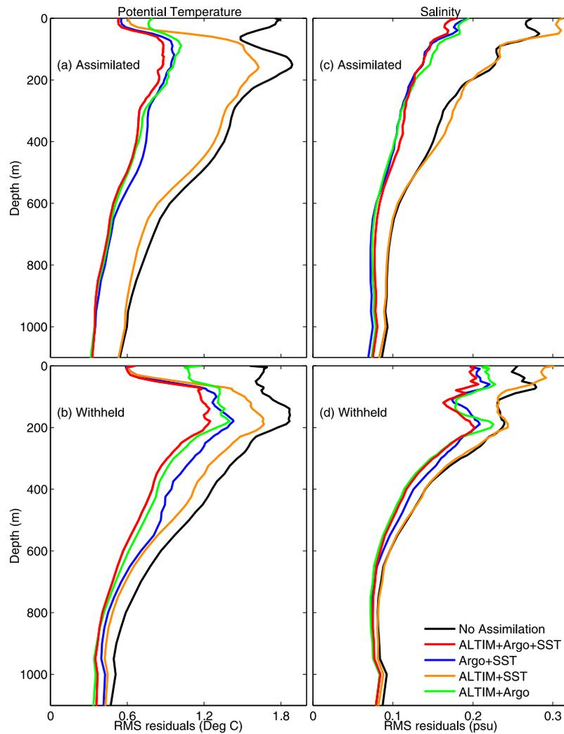
**Figure 3.** RMS residuals between observed and modelled (a, b) potential temperature and (c, d) salinity, using assimilated (Figures 3a and 3c) and withheld (Figures 3b and 3d) observations for each OSE. Statistics are computed for the region 90–180°E and south of the equator using 3159 assimilated and 600 withheld Argo profiles for the period January–May 2006.
