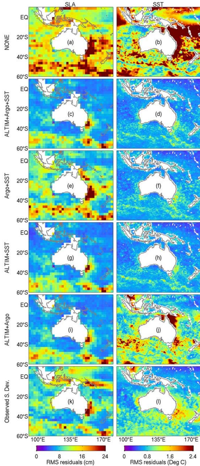
**Figure 2.** (a, b, c, d, e, f, g, h, i, j) RMS residuals between observed and modelled SLA (left column) and SST (right column) for each OSE; and (k, l) the observed standard deviation. Statistics are computed using atSLA observations from Jason, Envisat, and GFO (left column) and AMSR-E for the period January–May 2006.
