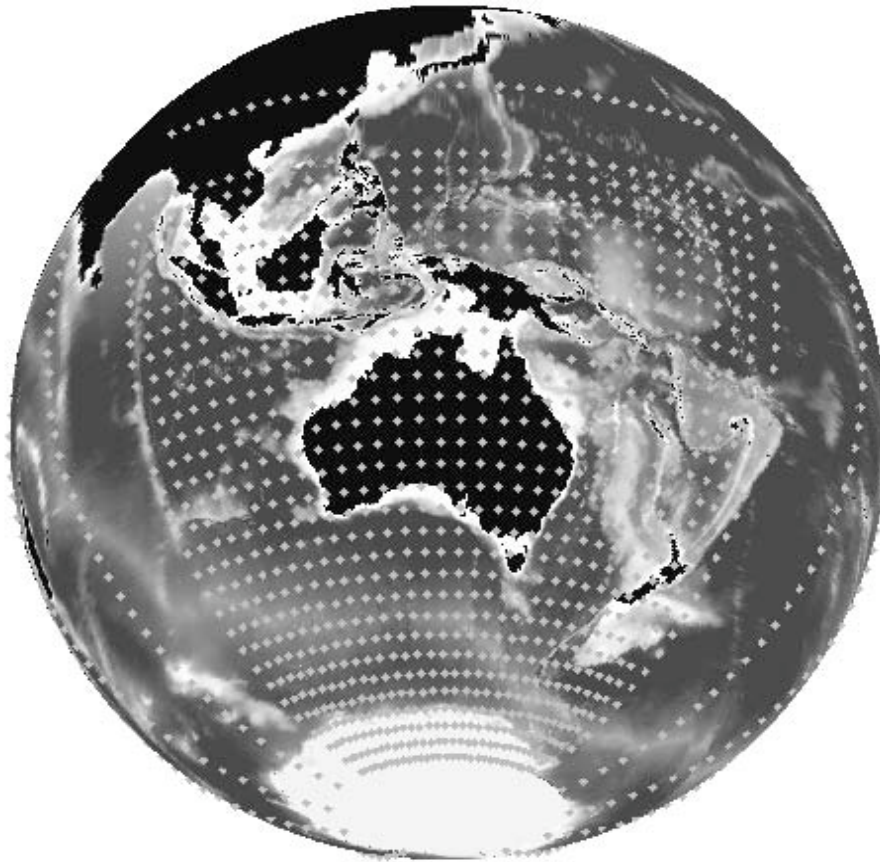
Figure 1: Ocean Forecast Australia Model horizontal grid. Water cells are coloured according to the depth of bathymetry, every 30th grid point is shown as a grey dot.
