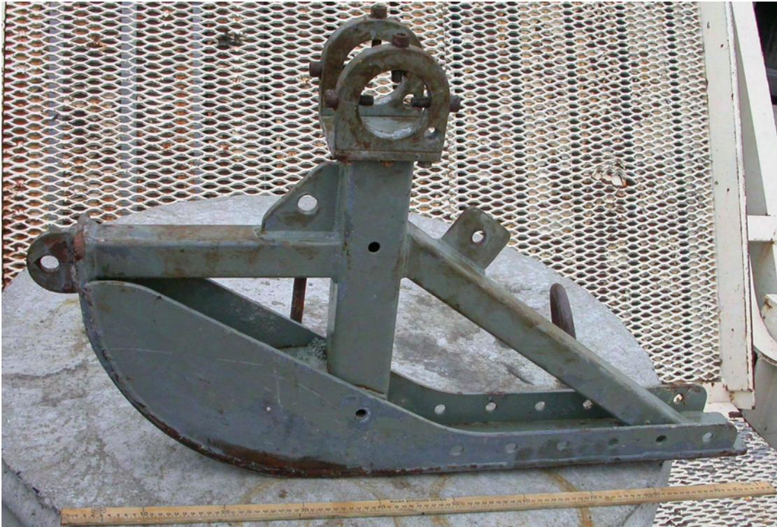
Figure 7: Dimensions of the beam trawl shoe.
