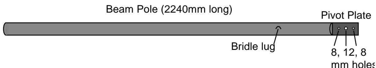
The pivot and breakaway bolts are stainless steel with the central pivot bolt of 12 mm and the break-away bolts being 8 mm diameter. It is recommended that one break-away bolt is used initially and the second one installed if the first breaks regularly. The pole should be positioned with the plate in the vertical plane as the main stresses appear to come from the tickler chains digging in trying to bring the shoes together as discussed above.
