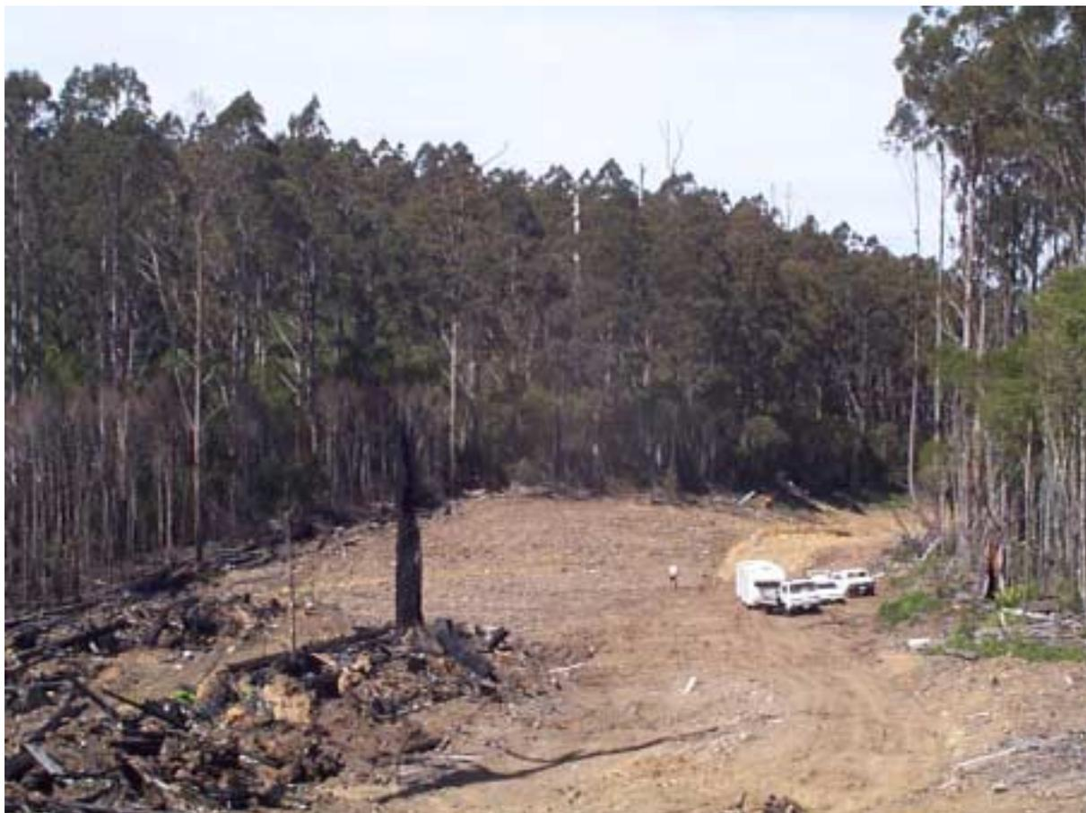
Figure 5. A view of the Tanjil Bren field site looking to the south west. The CAR lidar caravan is seen attached to the truck that carries the 240 V generator. Lidar signals were recorded mainly from the trees in the background, although some signals were recorded from the dead trees to the left and the tall trees on the right. Two levels of vegetation canopy can be seen. The taller trees are *Eucalyptus regnans* (Mountain Ash).
