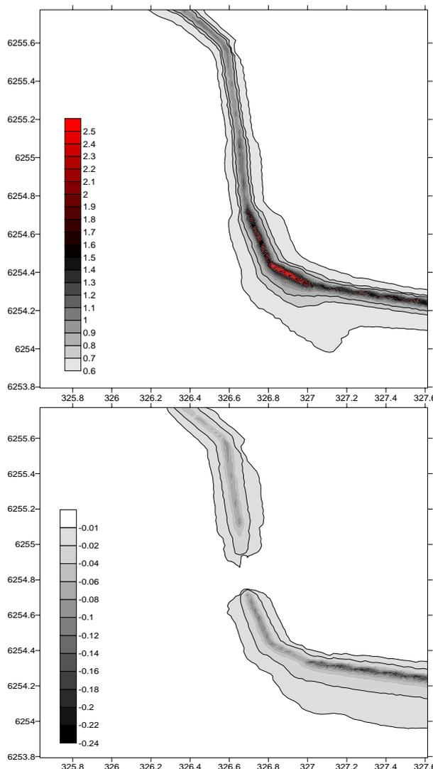
Figure 5. Predicted near-road 24 h CO concentrations (ppm) for a segment of Victoria Rd (see Figure 3). Top- base case; Bottom- difference between BTM and base case.
