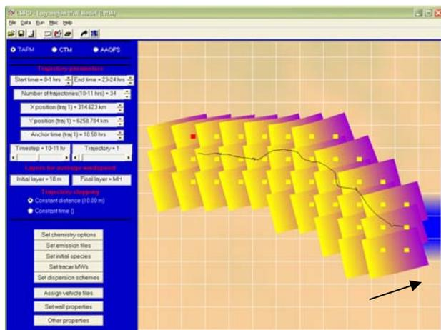
Figure 4. Showing the area covered by the Lagrangian Wall model for 34 trajectories which cover the length of Victoria Rd (line). The arrow indicates the direction in which the “walls” are moving for this particular hour. Each square represents a TAPM 2 x 2 km<sup>2</sup> urban cell.
