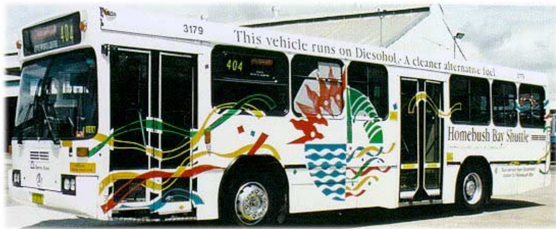
Figure 7.1 Diesohol bus used by Sydney Buses from 1993 to 1998.
