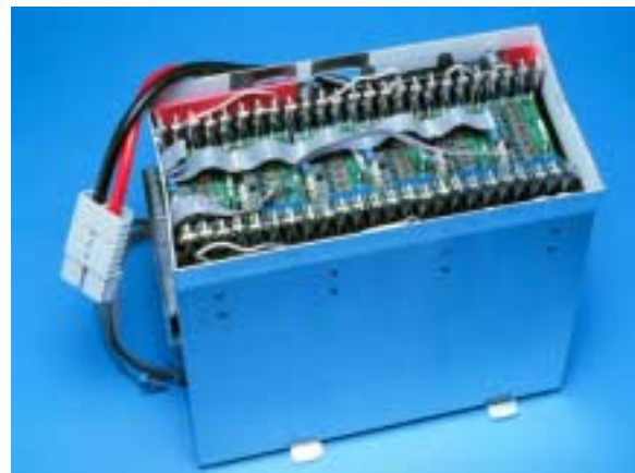
Figure 6: One Half of the Supercapacitor Pack
