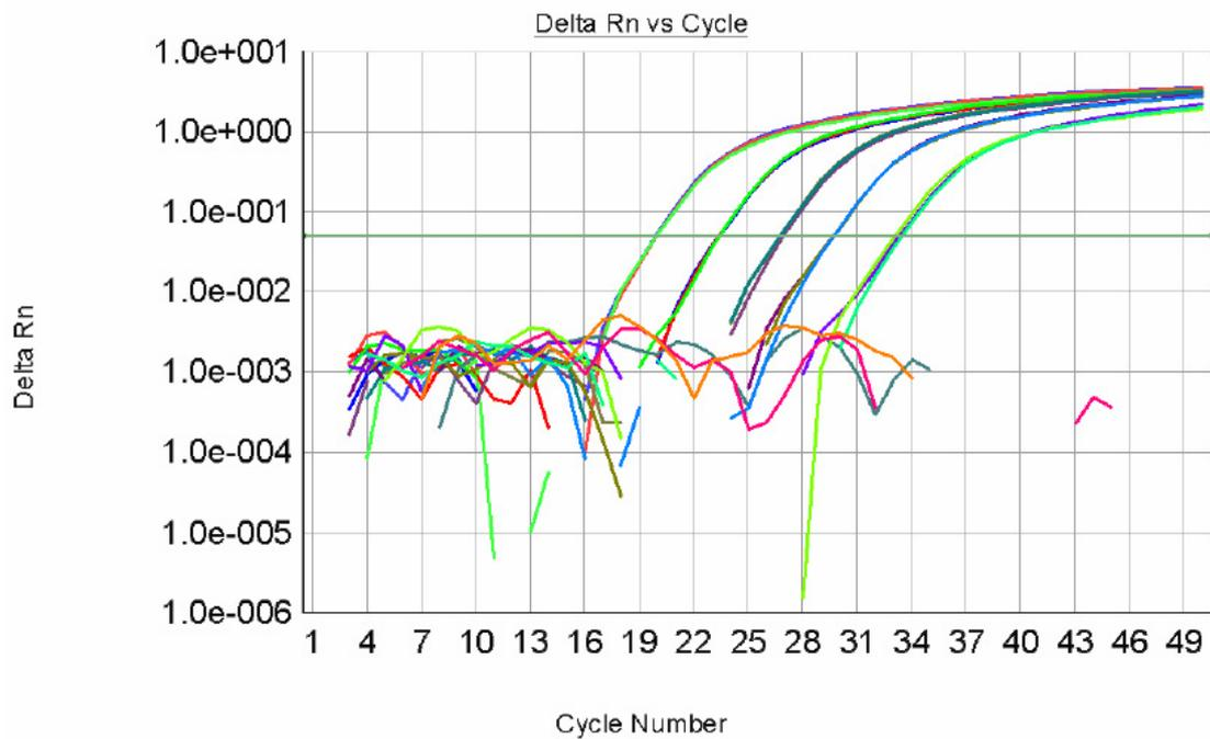
**Figure 20. Real-time PCR plots of standards (10-fold serial dilution), showing number of cycles necessary for concentration to reach the threshold (horizontal line).**
