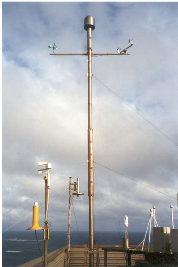
Figure 1. In situ view of the 10-m Cape Grim air inlet
