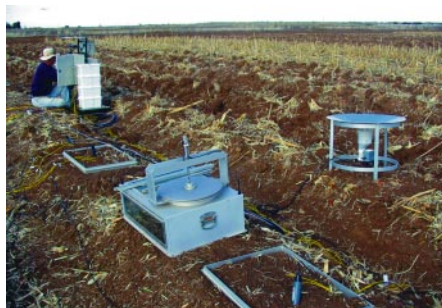
Instruments installed by CSIRO Atmospheric research in stubble near Griffith are measuring nitrous oxide emissions from maize.
