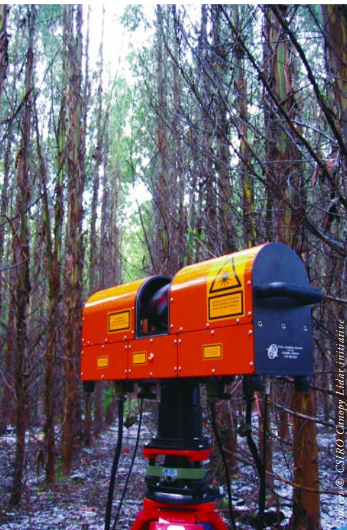
CSIRO's ECHIDNA™ in Tasmanian snow. The light-emitting instrument can measure forest canopies in poor weather conditions that would not be conducive to photographic measurements.
