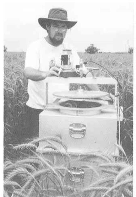
Mick Meyer monitors gas release and uptake in a wheatfield during OASIS.
