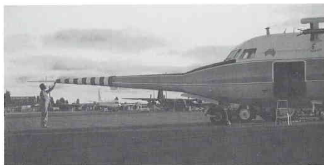
Dan Gogoasa checks the instrumented nose cone on the F27 research aircraft
