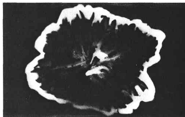
Ammonium nitrate particle after coating with nitron and silicon monoxide and exposure to water vapour.
