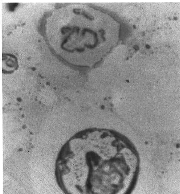
Particles containing sodium give a yellow colour with dipicrylamine; potassium gives a deep red.
