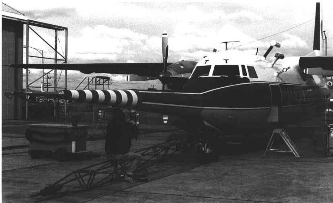
The F27 research aircraft being fitted with meteorological instruments in preparation for the Southern Ocean Cloud Experiment
