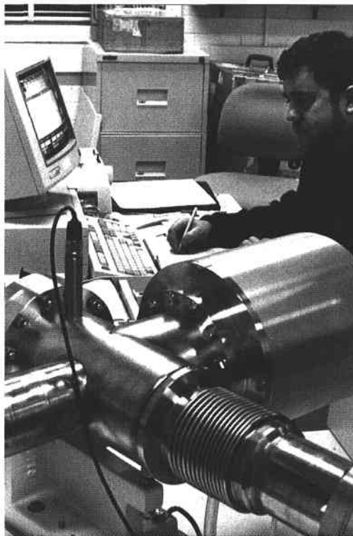
Colin Allison measures the isotopic make-up of carbon dioxide with GASLAB's mass spectrometer.
