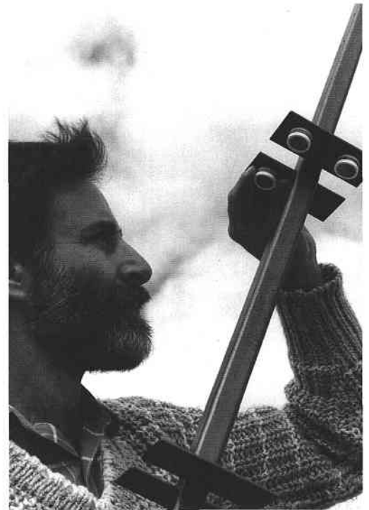
Greg Ayers installs a passive air sampler designed to measure levels of acidic compounds in the air.
