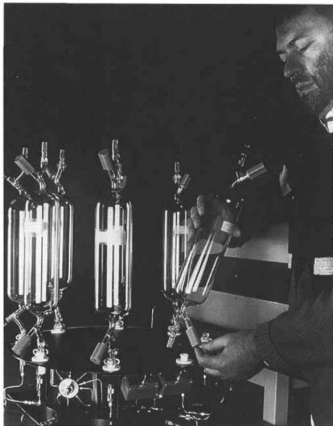
Dr Paul Steele prepares air flasks for chromatographic analysis in GASLAB.
