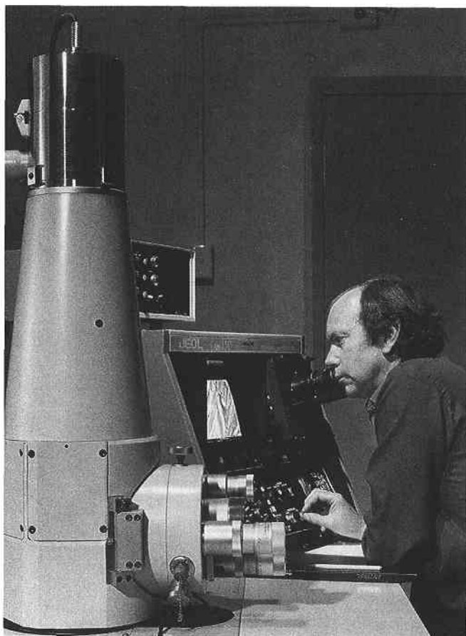
An electron microscope enables Dr John Gras to determine the size and nature of aerosol particles collected during a study of visibility reduction in Melbourne.
