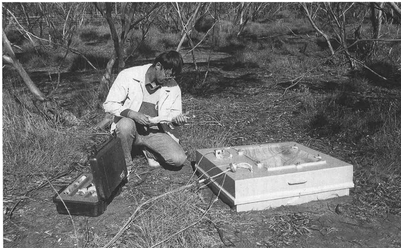
Professor Shang Shuhui, a visitor to the Division from the Institute of Applied Ecology in China, monitors the release of greenhouse gases from soil at a site in northern Victoria.
