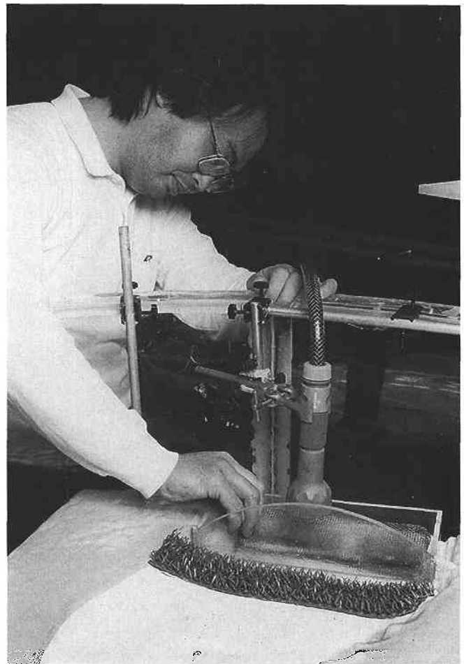
Dr Humio Mitsudera is studying ocean currents using a rotating tank. Water flowing into the tank models the wind-driven currents flowing through Bass Strait into the Tasman Sea.
