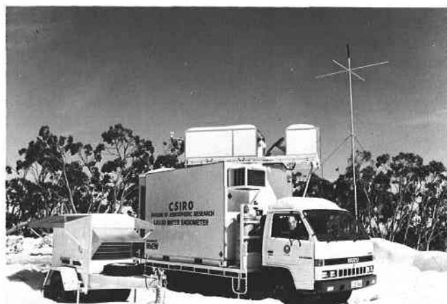
*The radiometer, constructed at the Division for the Second Australian Winter Storms Experiment*
