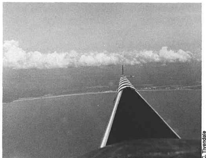
*The instrumented nose cone of the CSIRO F27 — used to obtain data about tropical cyclones. Turbulence vanes measure air motion.*
