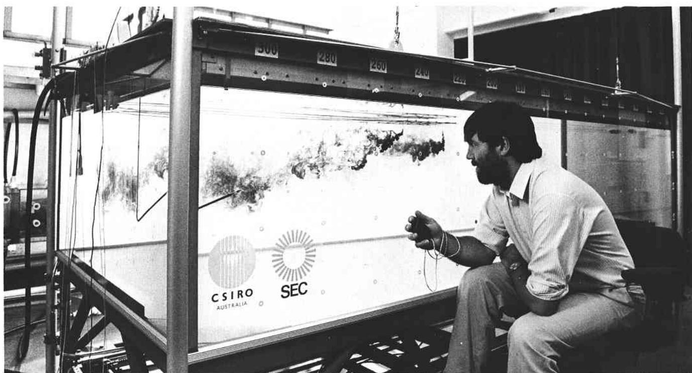
*The behaviour of smoke plumes in the atmosphere is studied in this 4000 litre modelling tank. Saline solutions are used to generate the buoyancy flux normally produced by heat.*
