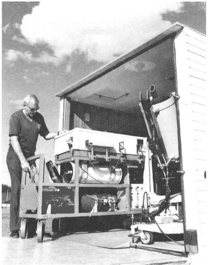
The Division's CO 2 and ruby lidars are now housed in a caravan, which enables the scientists to take them off the site for field expeditions. Recent expeditions were to Mildura (October, 1984 and July 1985) and to the Latrobe Valley (March, 1985).
