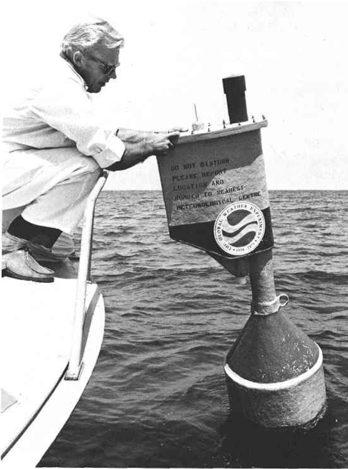
Fig. 6. Launching one of the southern hemisphere's 300 drifting buoys in the International GARP Experiment. Moving with the ocean currents, the buoys measure sea-surface temperature and pressure. The information is transmitted by radio to Toulouse, France, via the Tiros-N and NOAA-6 satellites which also fix the buoys' position at regular intervals. The buoys move in a generally easterly direction and typically have useful life spans of a year plus before the batteries expire.
