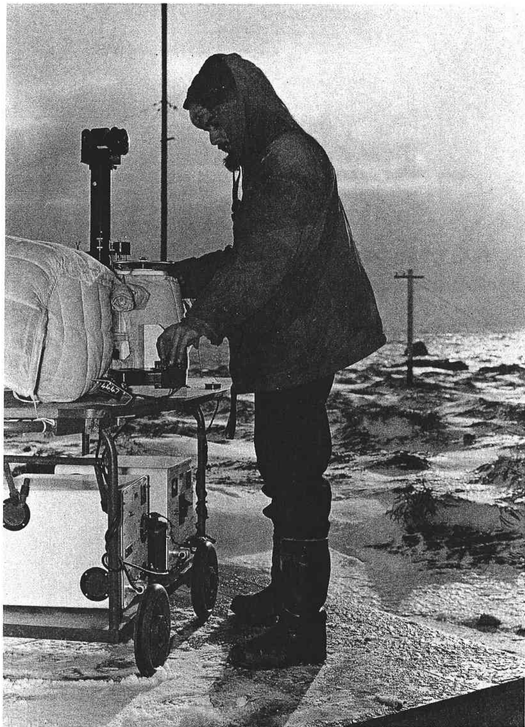
Macquarie Island - Using a Dobson Spectrophotometer to measure ozone in the upper atmosphere.
