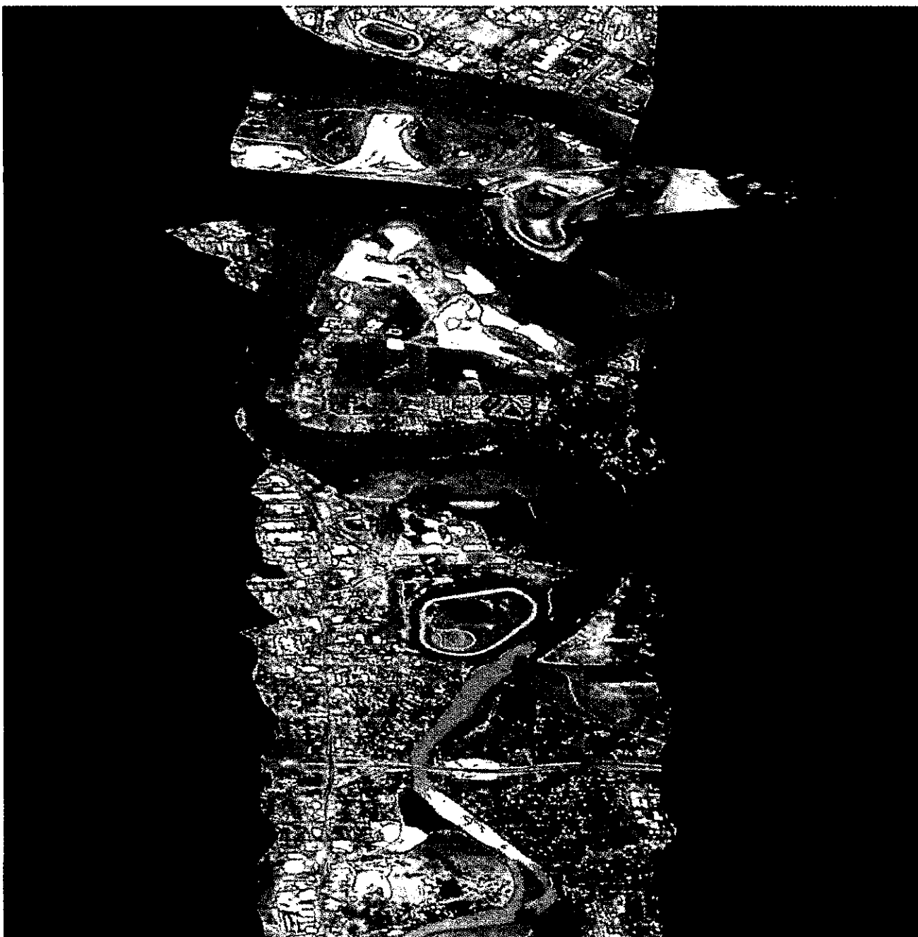
Figure 10: CASI image of the Swan River, using the best possible subset of spectral bands
