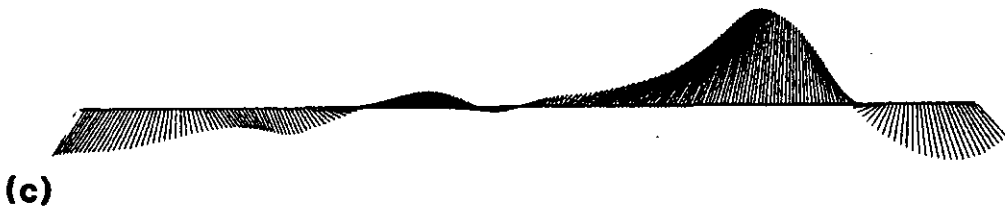
Fig. 9. (a) Temperature time series (each mark is a day) from an Aanderaa current meter. (b) Current vector time series ("stick diagram"); each line is an hourly current vector indicating strength and direction. The speed scale is as shown. (c) Filtered vector time series, to eliminate short-term variations. Same scale as for (b).
