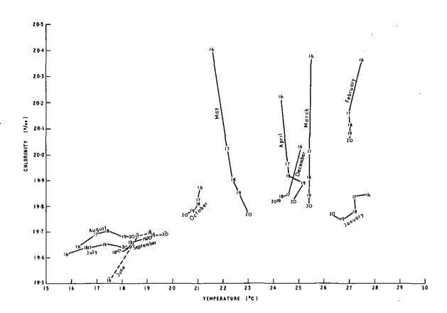
Fig. 2. - Temperature-chlorinity diagrams for northern section, July 1968 to June 1969 (November, no data). Numerals indicate coordinates of mean T-Cl value for each station (16-20).
