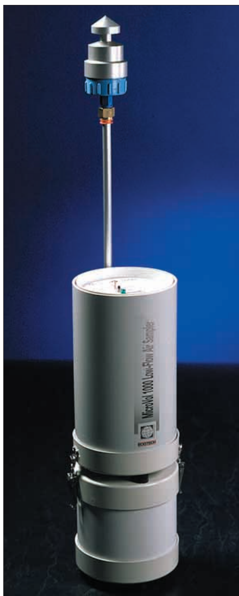
Ecotech's Microvol particle sampler, which collects particles and selected gases for subsequent analysis. The instrument has been developed from a CSIRO prototype.
