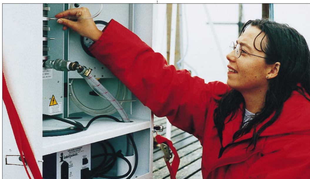
Rebecca Webb, from the University of Tasmania, adjusts the aerosol sampler flow rate on the roof of the Cape Grim station.
