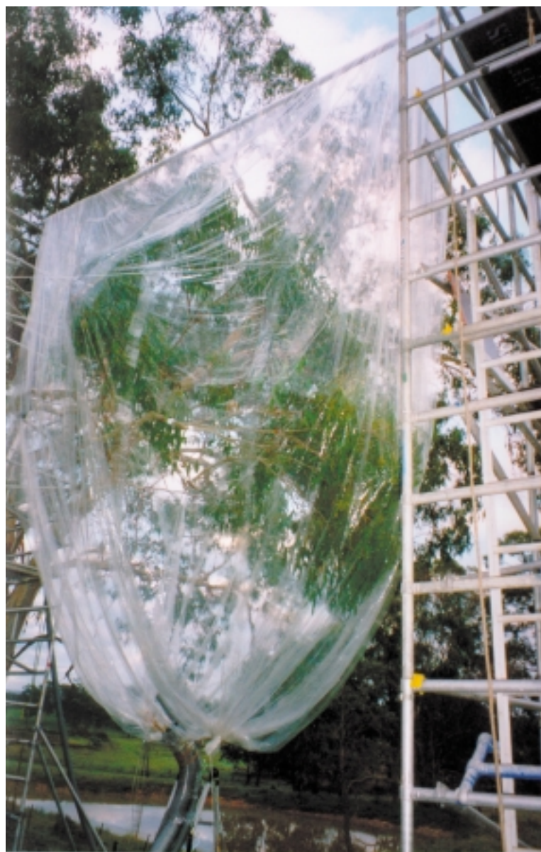
Measuring hydrocarbon emissions from plants. Emissions are collected in a teflon film bag.
